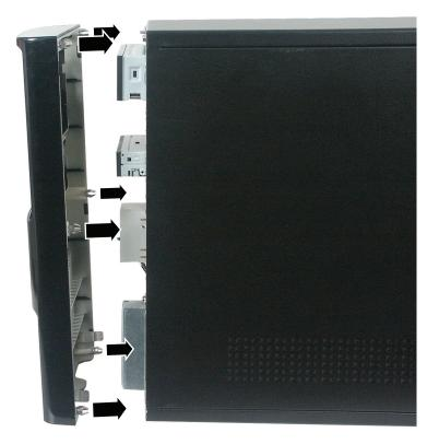
**2** Press the bezel firmly into place.
